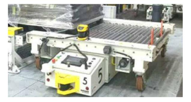
Automatic Guided Vehicles (AGVs) have come a long way in the past few decades since the 1977 Raymond Electote. Getting used to driver-less cars now is not much different than it was with driver-less vehicles in the manufacturing and distribution environments years ago. Today's AGVs are reliable and have proved themselves in industrial environments.
